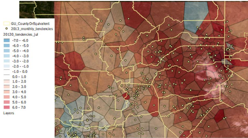
2013 July minus June difference (°C) in averaged 1400 PDT temperature. Actual range is -2.64 to +6.99 °C. Based on observations from mesonet stations.
