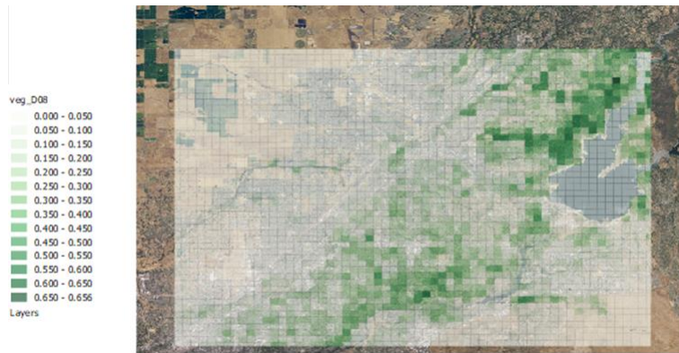
NLCD 2011-based calculations of canopy cover in D08 500 m domain
