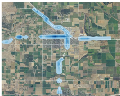
Figure 5-53: Change in near-surface temperature from vehicle electrification in the Woodland area. Example: 1700-PDT (rush-hour) average change in the interval July 1 – 15, 2013. Maximum average cooling is 2.2 °C (darkest blue).
