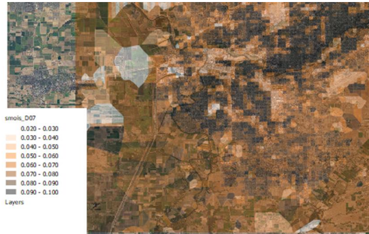
NLCD2011_GIRAS-based calculation of soil moisture content in D07 (500 m domain)
