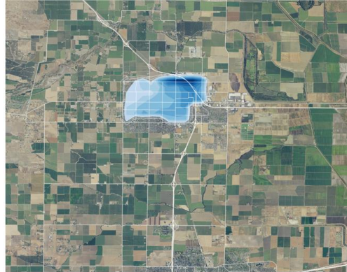
Figure 5-52: Change in air temperature from canopy in Woodland. Example: all-hour average change in the interval June 1 – 15, 2015. Maximum average cooling is 1.4 °C (darkest blue).
