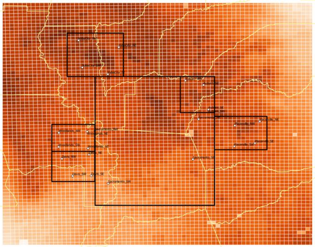
Figure 5-5: UHII-computation tiles and upwind reference points in the 6-counties Capital region (superimposed on a random-hour temperature field).
