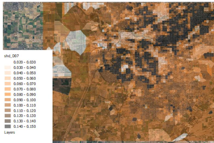
NLCD2011_GIRAS-based calculation of shdfac in D07 (500 m domain)
