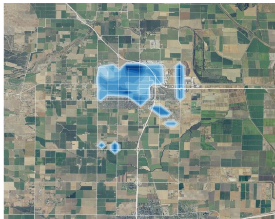
Figure 5-51: Change in roadway temperature from cool pavements in Woodland. Example: average changes at 1500 PDT, August 1 – 15, 2016. Maximum average cooling is 10.9 °C (darkest blue).
