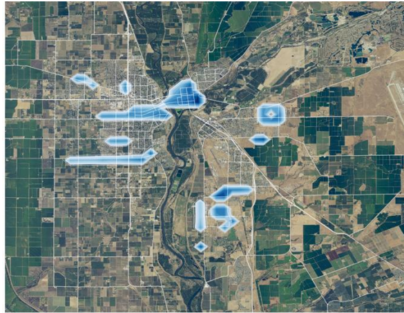
Figure 5-45: Change in urban-canopy air temperature from cool roofs and pavements in the Yuba City / Marysville area. Example: average changes at 1500 PDT, August 1 – 15, 2016. Maximum average cooling is 4.5 °C (darkest blue).
