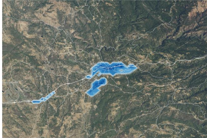
Figure 5-70: Change in urban-canopy air temperature from cool roofs and pavements in the Placerville – Diamond Springs area. Example: average changes at 1500 PDT, August 1 – 15, 2016. Maximum average cooling is 4.4 °C (darkest blue).
