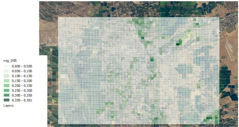
NLCD 2011-based calculations of canopy cover in D05 500 m domain 2-8.C
