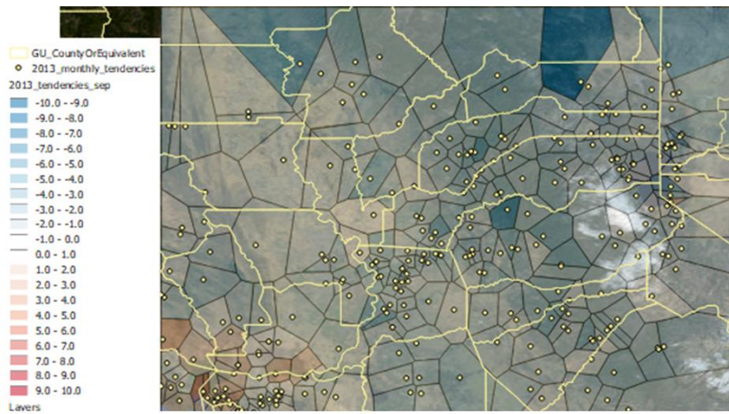
2013 September minus June difference (°C) in averaged 1400 PDT temperature. Actual range is -9.06 to +5.07 °C. Based on observations from mesonet stations.
