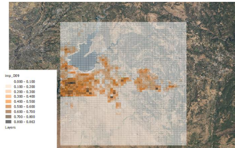
NLCD2011-based calculation of impervious cover: D09 500-m 2-10.E
