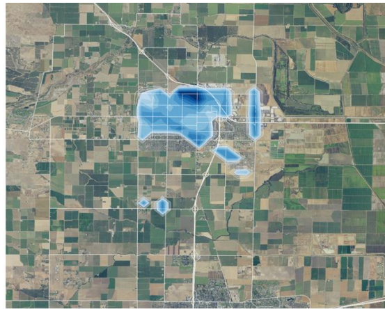
Figure 5-50: Change in urban-canopy air temperature from cool roofs and pavements in Woodland. Example: average changes at 1500 PDT, August 1 – 15, 2016. Maximum average cooling is 4.5 °C (darkest blue).
