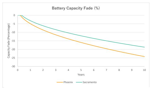
*Figure 5.* Average battery cell capacity fade over 10 years for a 200-mile EV with identical driving and charging cycles in Phoenix and Sacramento. Modeled from NREL's BLAST-V Lite tool.
