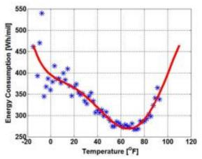
*Figure 1.* Nissan Leaf energy consumption per mile versus air temperature, using FleetCarma data. Source: Yuksel and Michalek.
