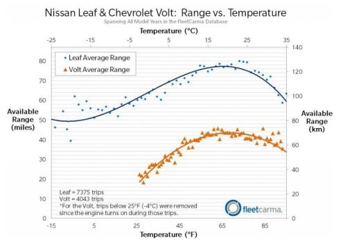
*Figure 3.* Chevrolet Volt and Nissan Leaf range and temperature, based on FleetCarma data.
