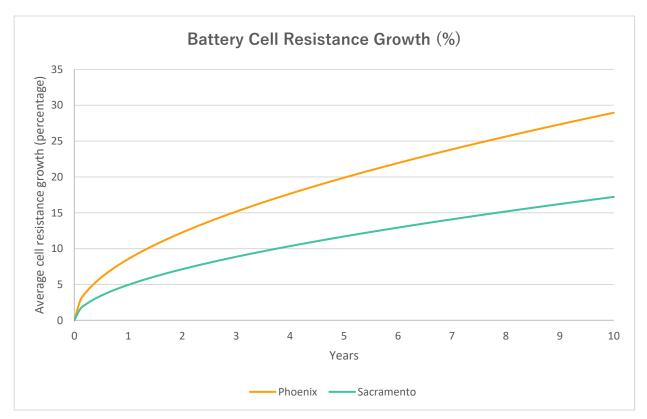
*Figure 6.* Battery cell resistance growth over 10 years for a 200-mile EV with identical driving and recharging cycles in Sacramento and Phoenix. Modeled from NREL's BLAST-V Lite tool.
