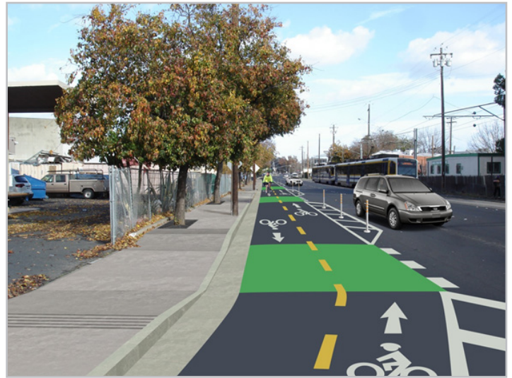
Figure 30: North 12th Proposed Two-Way Class IV Bikeway
