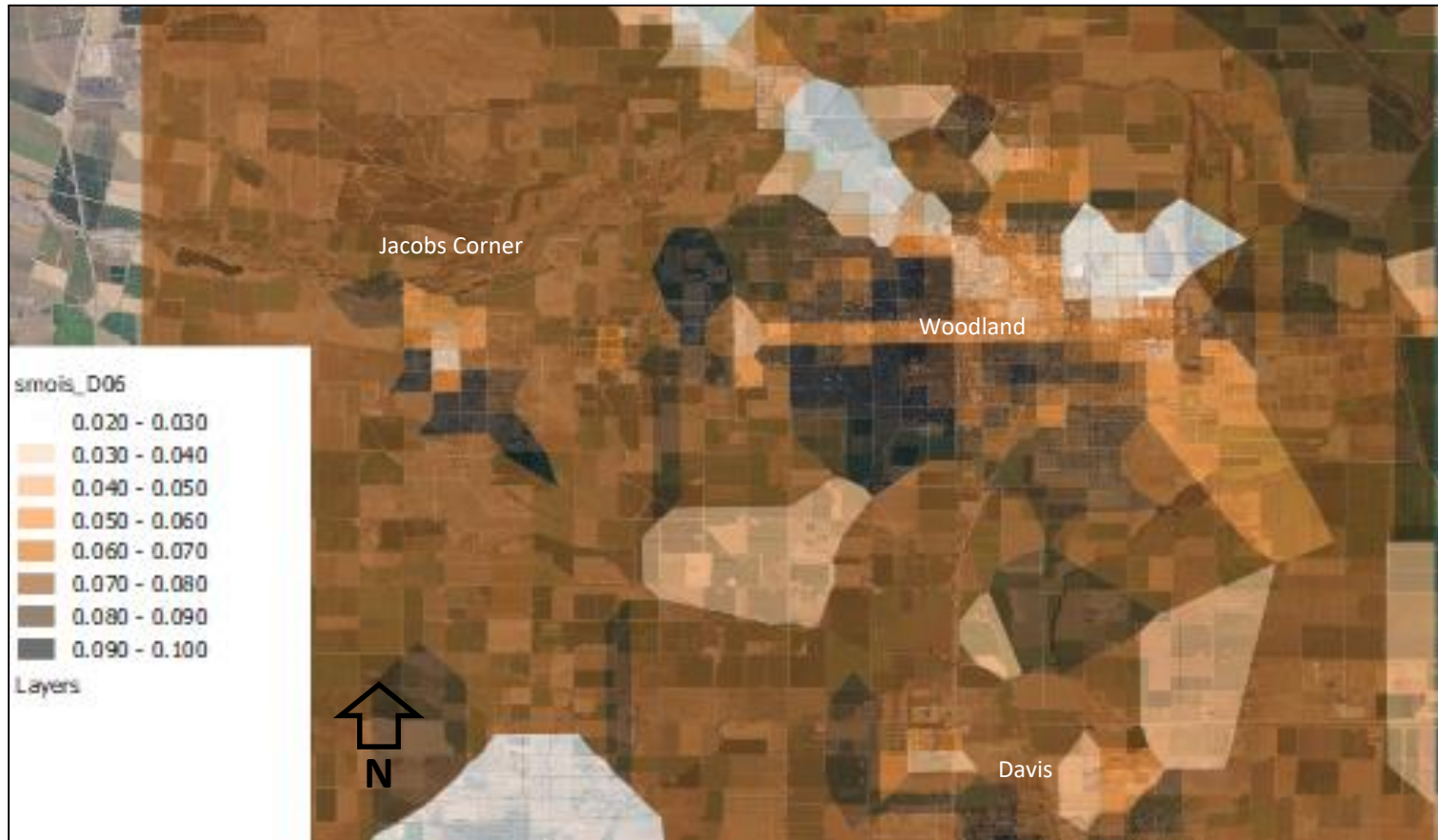
NLCD2011_GIRAS-based calculation of soil moisture content in D06 (500 m domain)
