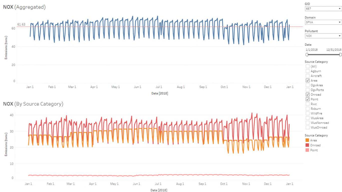
Figure B-30: Example timeseries plot for daily 2018 NO x emissions from area, on-road, and point sources for Sacramento Nonattainment Area
