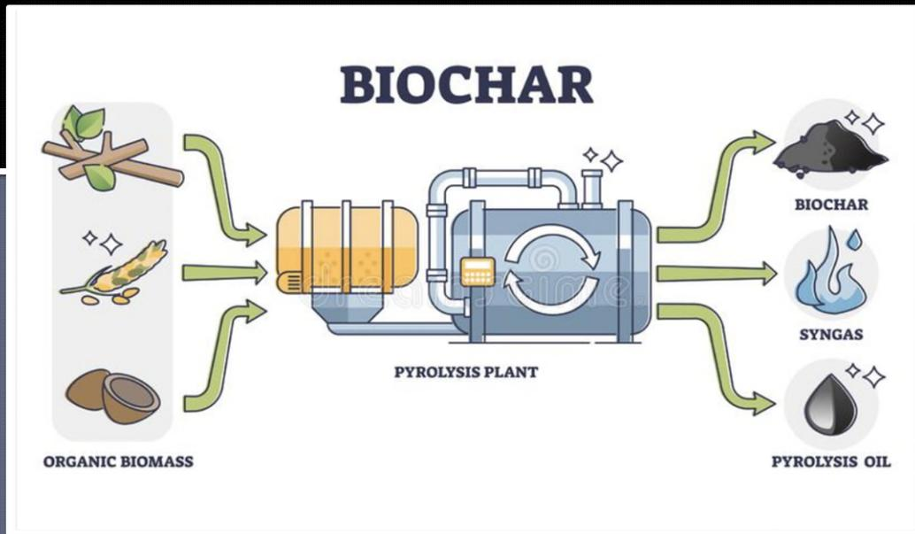
Biochar is created using pyrolysis when biomass is *heated, not combusted*, at high temperature in low oxygen environments. Other by-products are also produced during production depending on the type of system, including renewable energy in the forms of heat and syngas and bio-oils that can be used by ag or industry.
