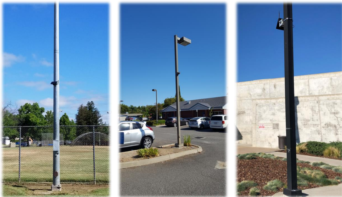
Figure 4-2. Deployed Clarity Node-S monitors.
