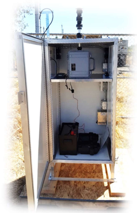
Figure 4-5. Phase 2 monitor stand-alone unit at the Veterans of Foreign Wars Post 1267 site.
