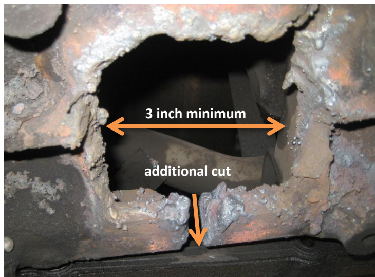
Sample of engine hole and cut to oil pan
